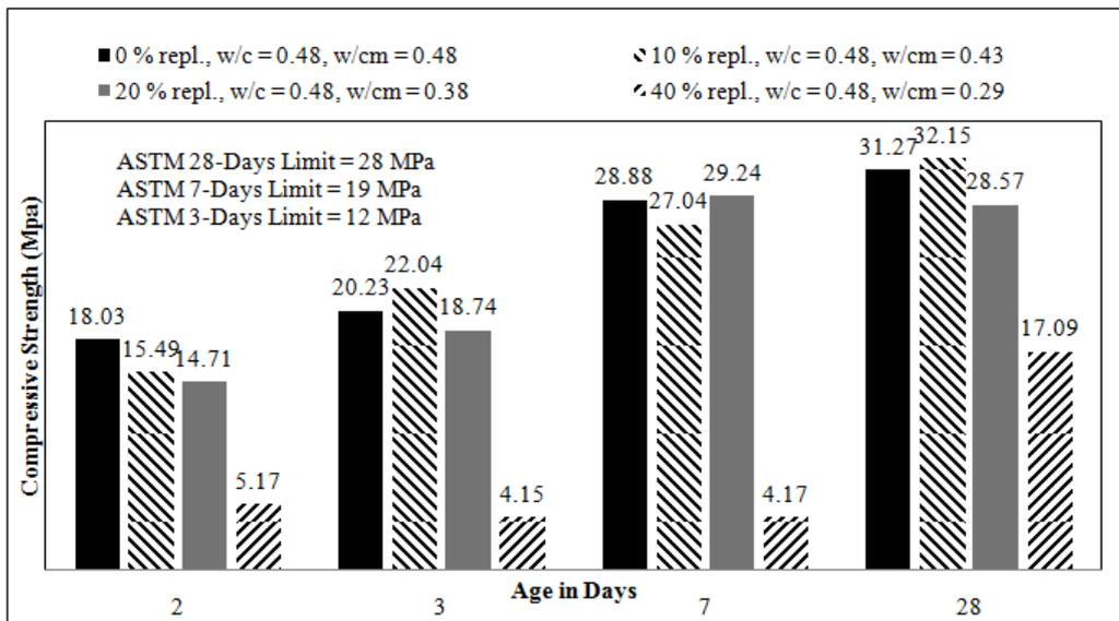
Fig. 2. Compressive strength for different cement/sludge mixes of constant w/c ratio 0.48 and varying w/cm
