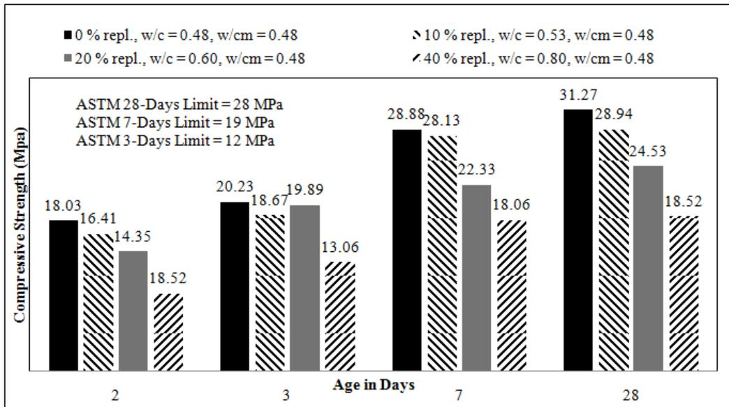
Fig.1. Compressive strength for different cement/sludge mixes of constant w/cm ratio 0.48 and varying w/c
