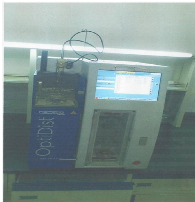
Fig. 2.1. Distillation apparatus assembly using electric burner
