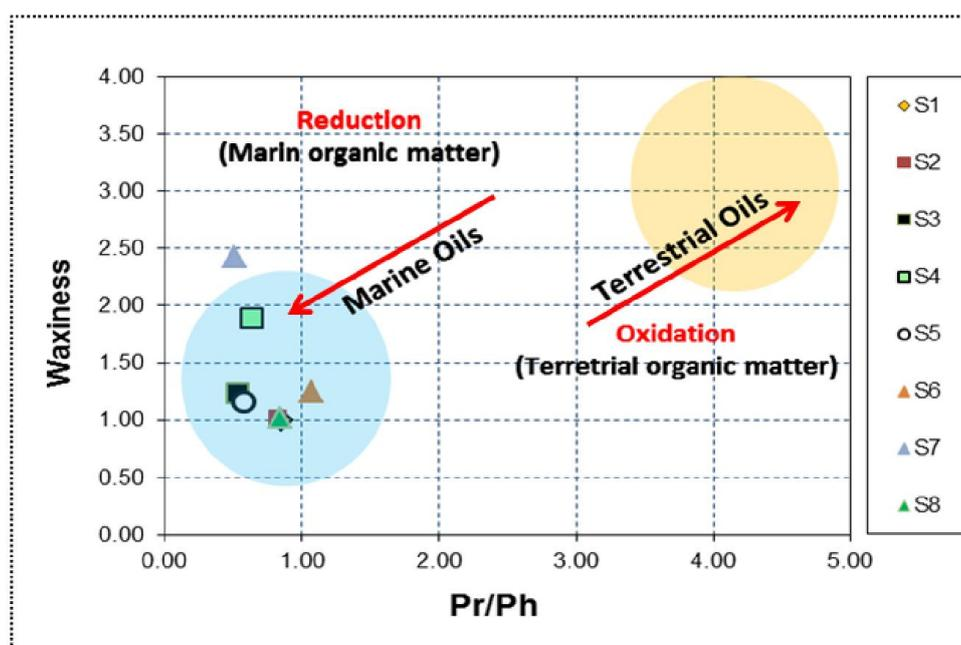
Figure 7. Cross plot of Pr/Ph vs. Waxiness of the studied oil samples
