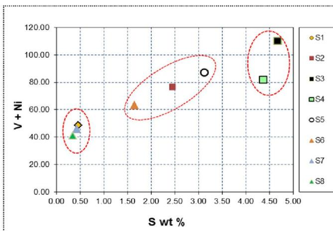
Figure 3. Cross plot of total concentration of (V+Ni) and sulfur contents
