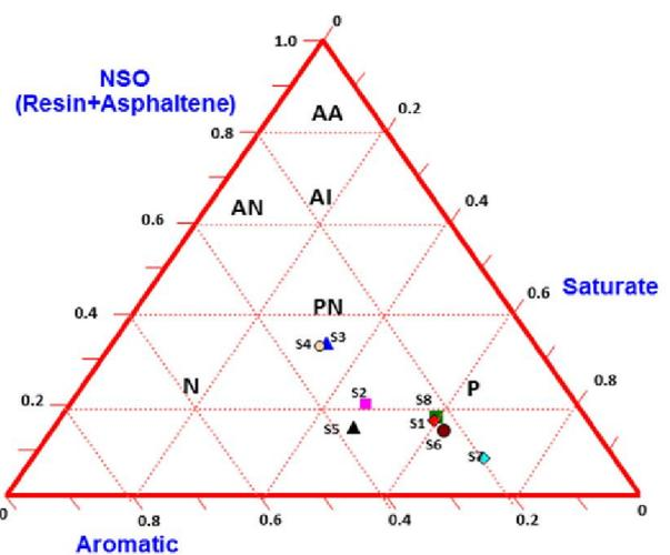
Figure 4. Ternary diagram between saturates, aromatics and NSO + asphaltenes showing types of crude oils in Gulf of Suez. P: Paraffinic; PN: Paraffinic Naphthenic; N: Naphthenic; AA: Aromatic Asphaltic; AI: Aromatic Intermediate and AN: Aromatic Naphthenic. Normal Paraffins Distribution and Isoprenoids (Pristane [Pr] and Phytan [Ph]) Parameters
