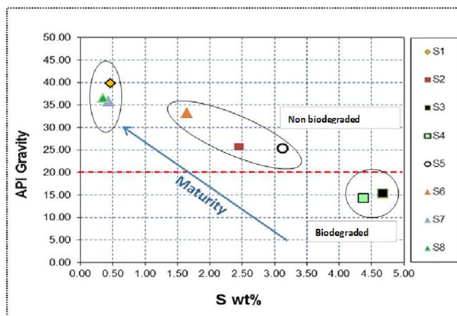
Figure 2. Cross plot of API gravity and sulfur contents
