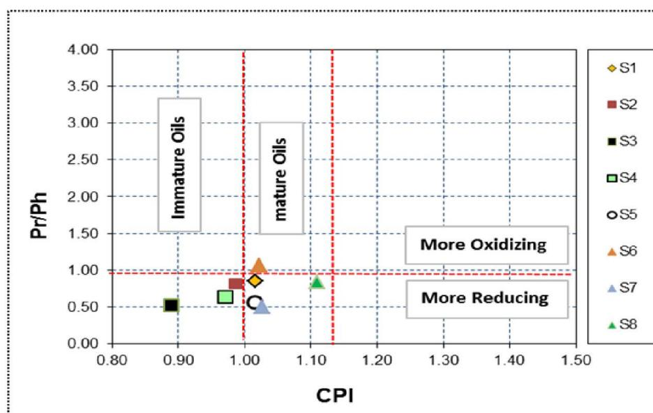
Figure 8. Cross plot of CPI vs. Pr/Ph of the studied oil samples
