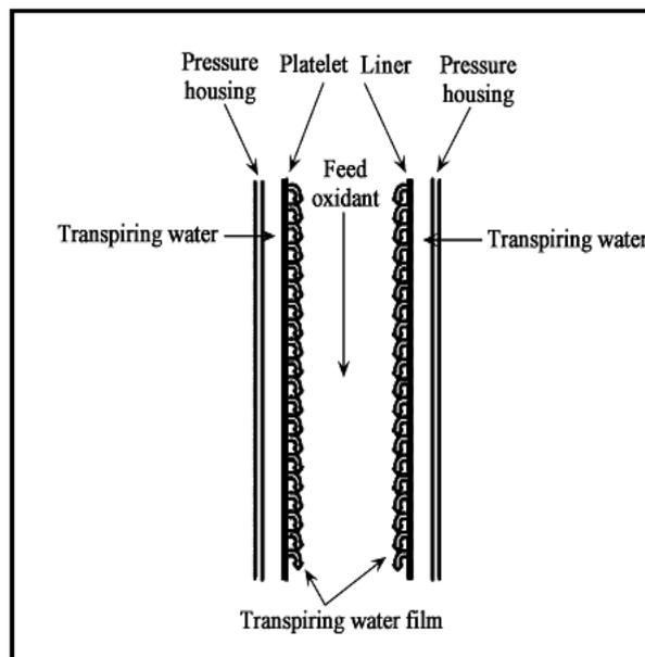
**Fig 3. Transpiring Wall Reactor (Veriansyah et al., 2007)**
