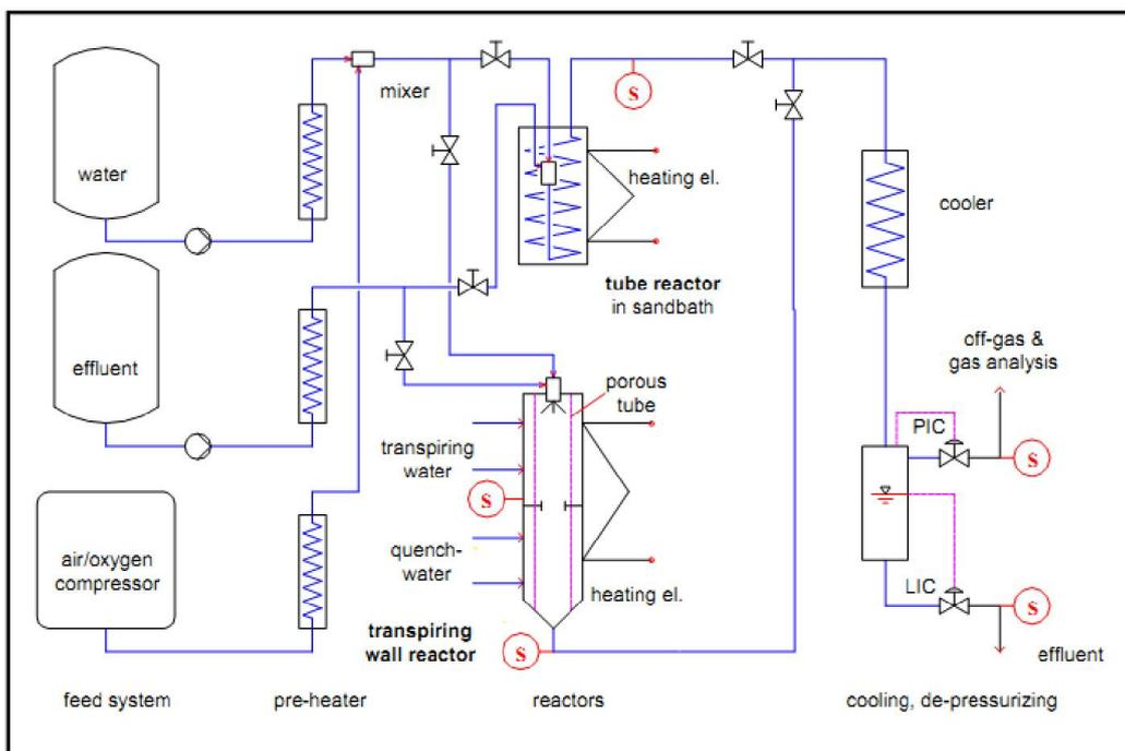
**Fig.2. Flow diagram of the SCWO Bench Scale Apparatus (3)**
