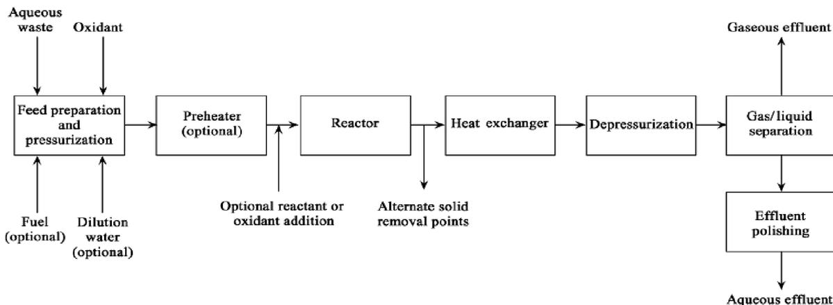
**Fig.1. Block flow diagram of typical SCWO process (Veriansyah et al., 2007)**
