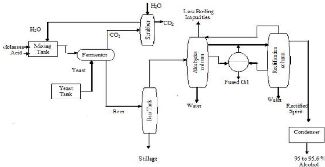
**Figure 1. Process Flow sheet of Alcohol Manufacturing**
