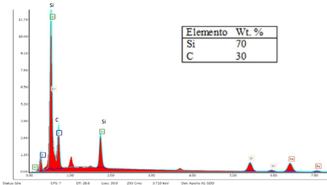
Figure 3. Chemical analysis of SiC obtained by the technique EDS
