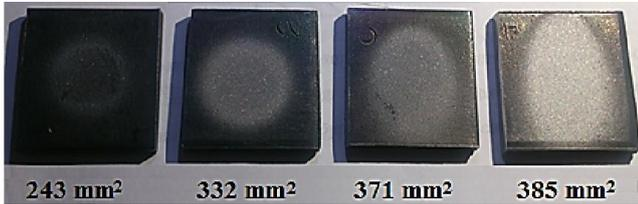
Figure 11. Traces generated by particles of SiC on SiC coating at an angle of impact: a) 90, b) 60, c) 45, d) 30 °
