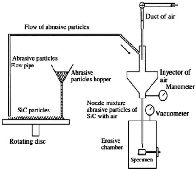
Figure 6. Schematic eroding prototype
