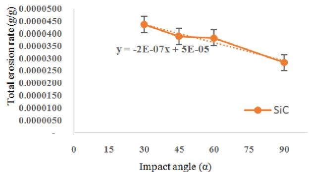
Figure 10. Graph of erosion rate of the coating of SiC
