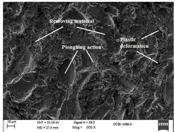
Figure 9. a) Damage from erosion coating  $30^\circ$
