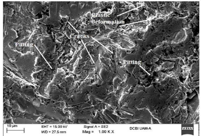
Figure 8. a) Damage by erosion of the coating at  $90^\circ$
