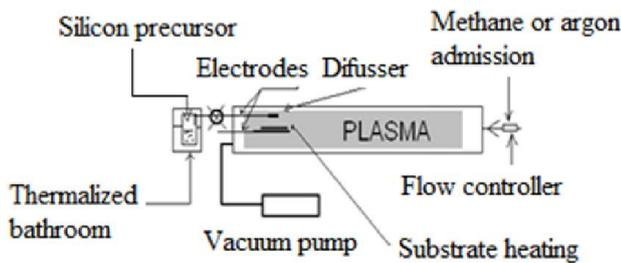
Figure 1. Schematic of the plasma CVD reactor
