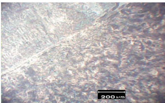
Fig 5.3. Weld interface to SS 304 (100X)
