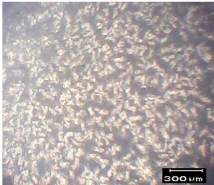
Fig 5.2. Corten steel BM (500X)
