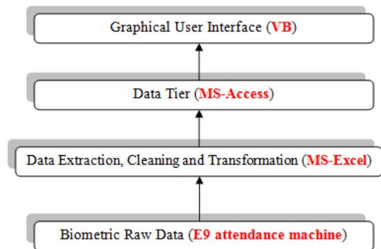
Figure 9. Multi-Tier Application Architecture
