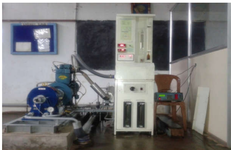
Plate 1. Computerized diesel engine test rig with exhaust gas analyzer
