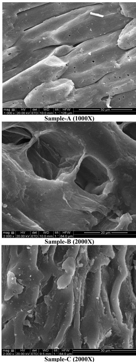
**Figure 10. SEM image of fracture surface of different sized Arecanut husk samples in Alkaline hydrolysis Pretreatment**
