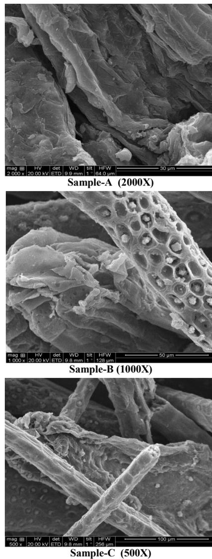
Figure: 9. SEM image of fracture surface of different sized Arecanut husk samples in Acid hydrolysis Pretreatment
