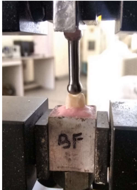
Figure 2. Tooth sample mounted in Instron 3382
