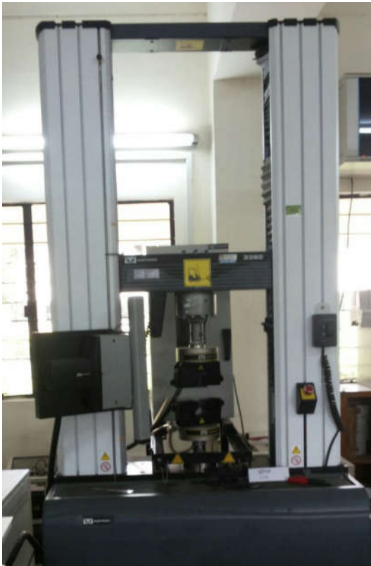
Figure 1. Instron 3382 (universal testing machine, USA)
