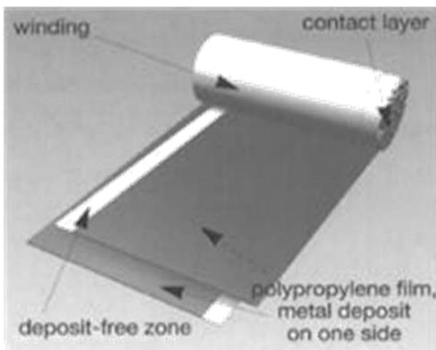
**Fig. 1. Metallized Polypropylene Film**
