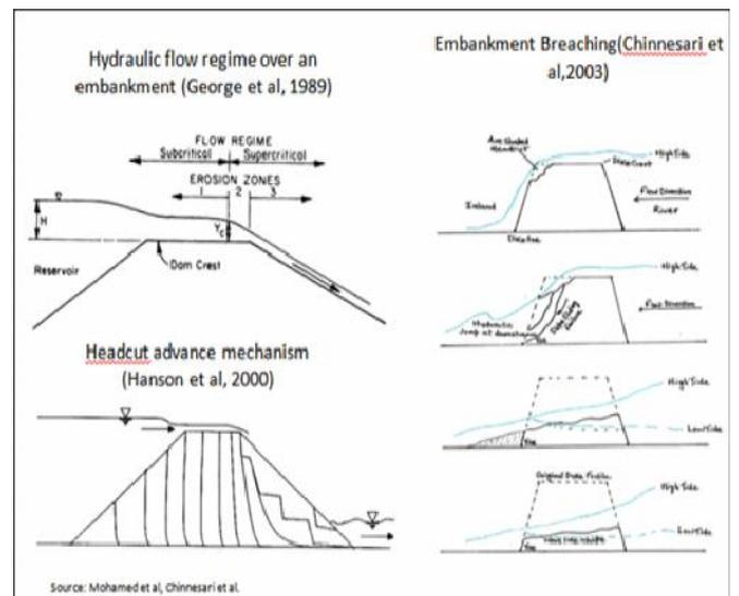
Fig. 1. Models of embankment breaching
