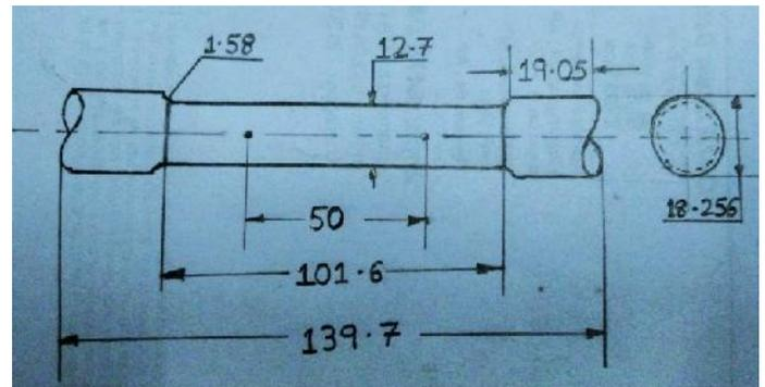
**Fig. 5. Drawing of Tensile Test Specimen**
