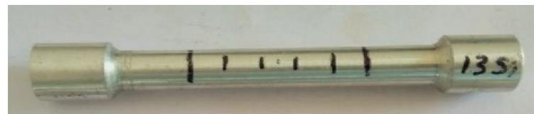
**Fig. 6. Photograph image of Tensile Test Specimen**
