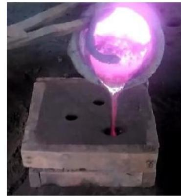
**Fig. 4. Molten Al-Si Alloy pouring into Sand Mold**
