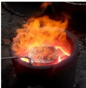
**Fig. 3. Heating Aluminum Alloy**
