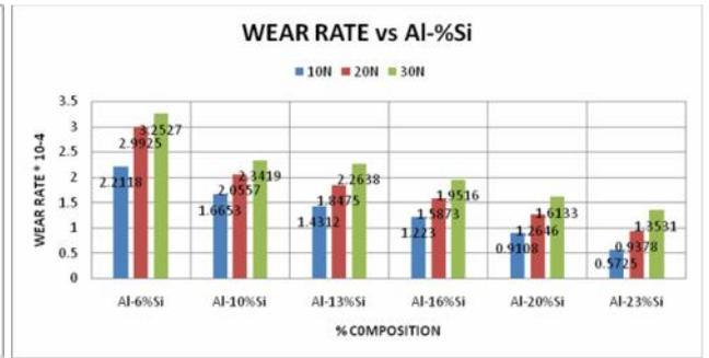
Fig. 19. Wear Test values of different Al-%Si alloy compositions
