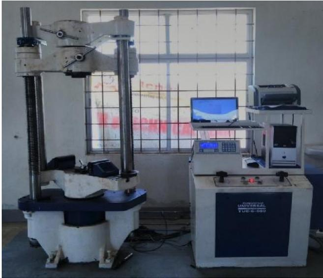
Fig. 7. Universal Tensile Testing Machine
