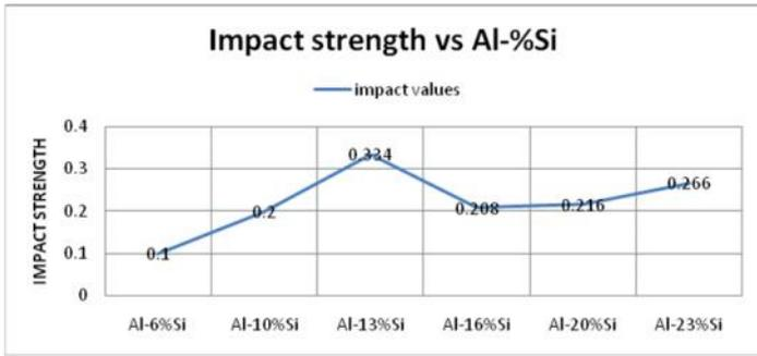
Fig. 18. Toughness values of various Al-%Si alloy compositions
