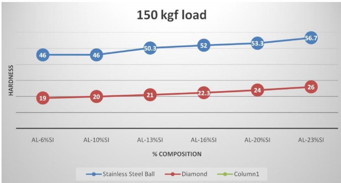
Fig 17. Hardness Values for 150 kgf load
