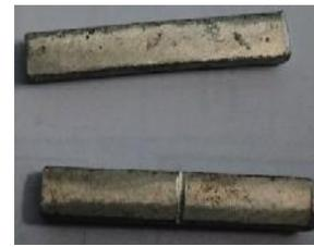
Fig. 9. Impact Test Specimen
