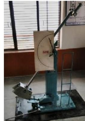
Fig. 10. Charpy Testing Machine
