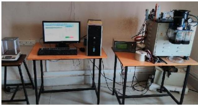
Fig. 11. Ducom friction and wear monitor pin on disc wear test machine
