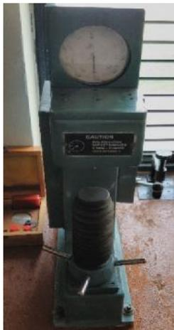
Fig. 8. Rockwell Hardness Testing Machine
