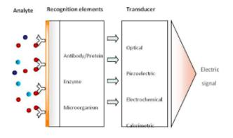
Current used biosensors are electrochemical type. Electrochemical biosensors are highly sensitive and easy to maintain. These biosensors have a low cost. Amperometric glucose biosensor is currently available in these days. Amperometric biosensor generate current when electrons are exchanged between electrode. Glucose of diabetic patient can be measured by using three enzymes.
