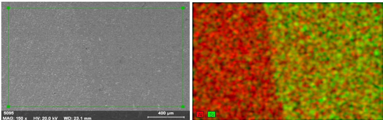
**Fig.1. SEM microstructure of weld region of T0 treated specimen and its elemental mapping**
