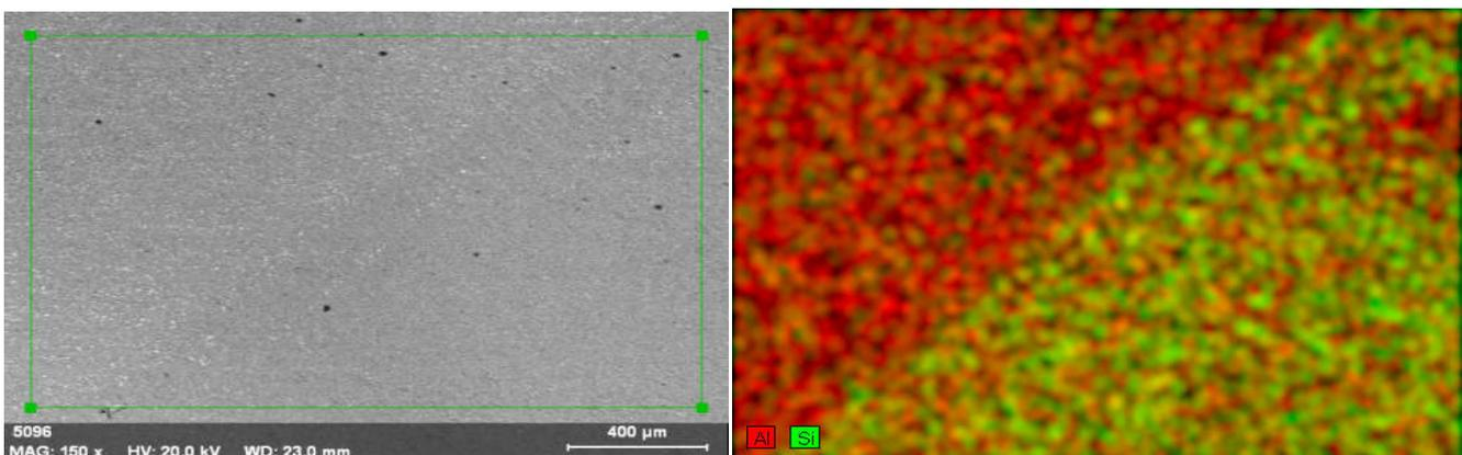
**Fig.2. SEM Microstructure of weld region of T6 treated specimen and its elemental mapping**
