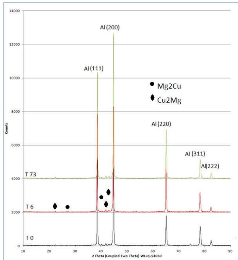
Fig.4. XRD Analyses from after T0, T6 and T73 heat treatments
