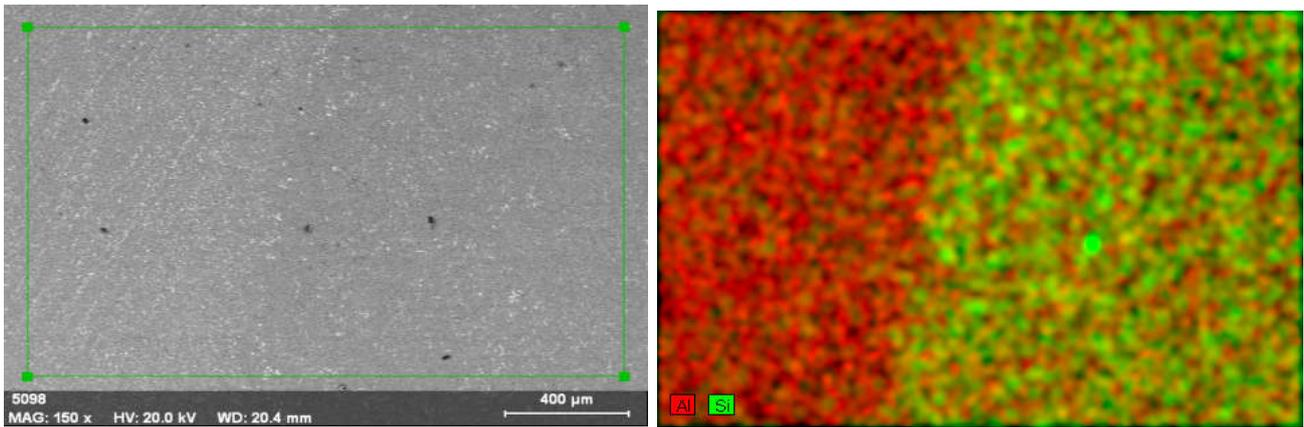
Fig.3. SEM microstructure of weld region of T73 treated specimen and its elemental mapping
