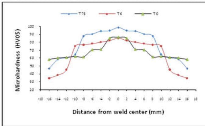
Fig.5. Microhardness of the welded regions with different heat treatments
