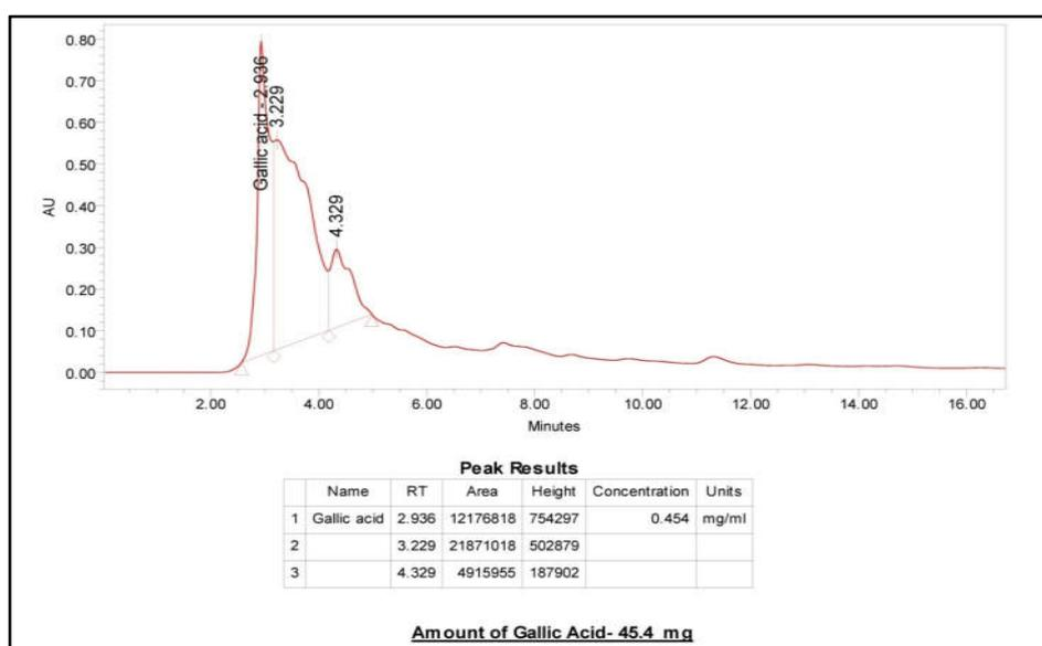
Fig. 5. Quantification of bioactive phenolic compound (gallic acid) in chitosan treated cell culture by HPLC method
