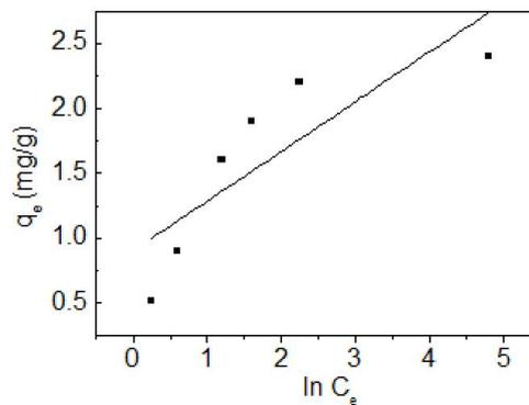
Figure 7. Temkin isotherm for sorption of Pb (II) ion by Corn husk. 0.5g dry weight biomass with 25 mL of Pb (II) Solution. pH 4
