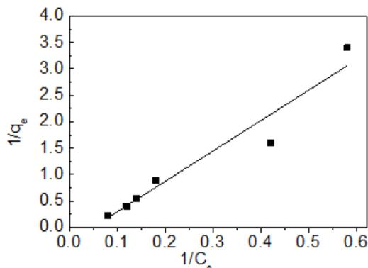
Figure 5. Langmuir isotherm for sorption of Pb (II) ion by Corn husk. 0.5g dry weight biomass with 25 mL of Pb (II) Solution. pH 4
