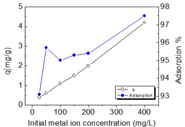
**Figure 2. Effect of initial metal ion concentration on biosorption of Pb (II) ions aqueous solution using Cornhusk. 0.5g dry weight biomass with25 mL of Pb (II) Solution. pH4**
