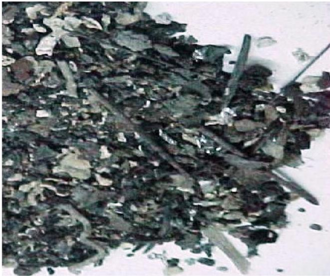
**Figure 8. Ash Particle Size between 0.5-4.75 mm**
