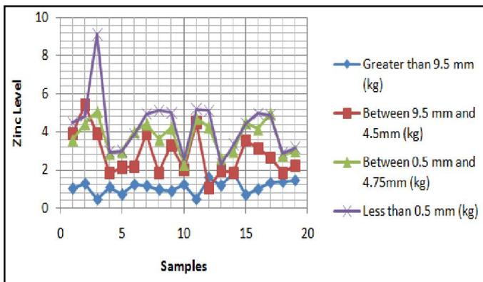
Figure 12. Samples Vs. Zinc Concentration as in EP Toxicity Test
