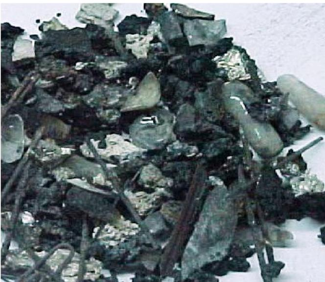
**Figure 9. Ash Particle Size between 4.75 – 9.5 mm**
