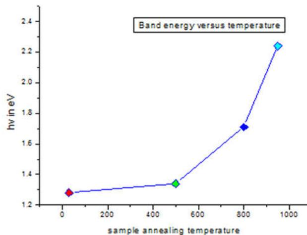
Fig.6. Band gap energy variation with the samples at varied annealing temperature of  $Fe_2Mn_2Ni_2Zn_2O_{11}$
