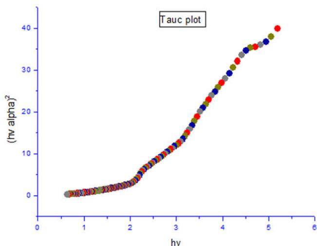
Fig. 5. The Tauc plot of  $Fe_2Mn_2Ni_2Zn_2O_{11}$
