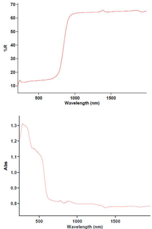
Figure 1. UV-VIS spectrum of  $Fe_2Mn_2Ni_2Zn_2O_{11}$  (reflectance & absorbance)
