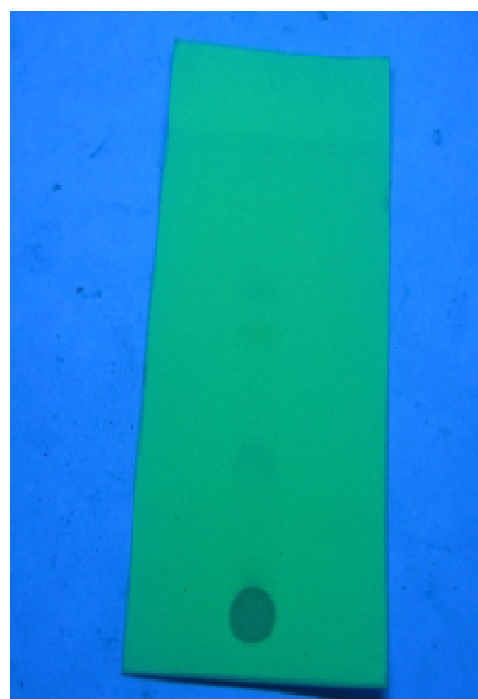
Figure 2. T.L.C. Plate in U.V. Fluorescence analyzer
