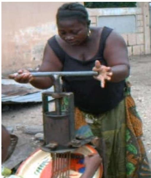
Figure 5. Kluiklui Extruder Prototyped tested by a User
