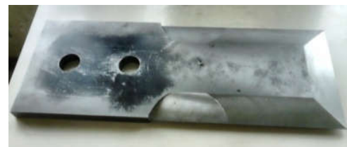
Figure 10. Rotary knife cutter after machined
