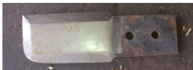
Figure 2. Rotary knife cutter at Sugar Factory Sei Semayang
