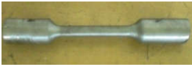
Figure 11. Tensile test specimens
