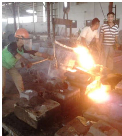
Figure 7. Pouring of Rotary knife cutter
