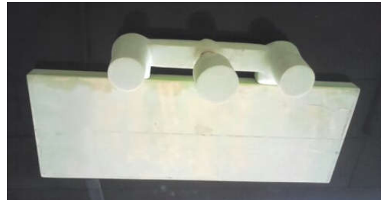
Figure 4. Pattern of Rotary knife cutter
