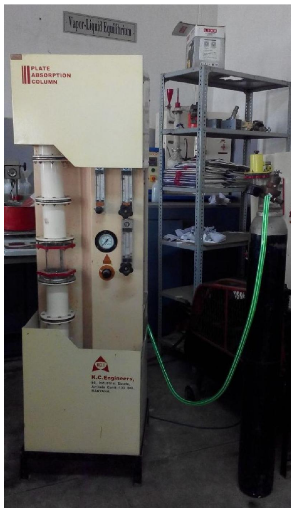
Figure 5. Overlook of Plate Absorption Column
