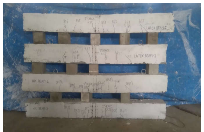
Figure 5. Crack pattern of test beam specimens
