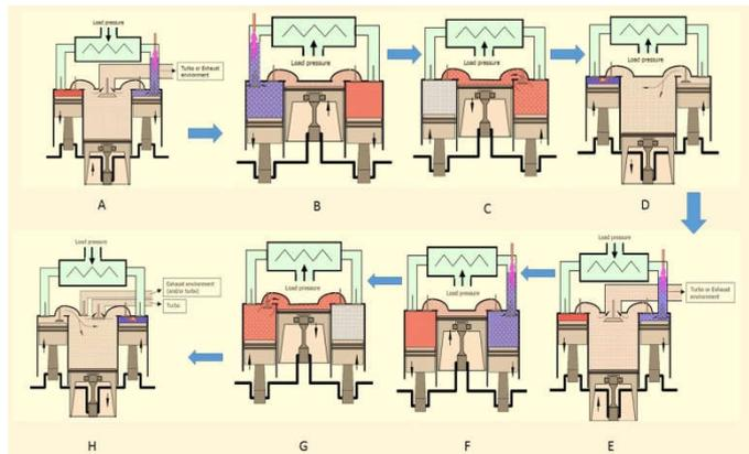
**Figure 2. Working cycle of 5 stroke engine**
