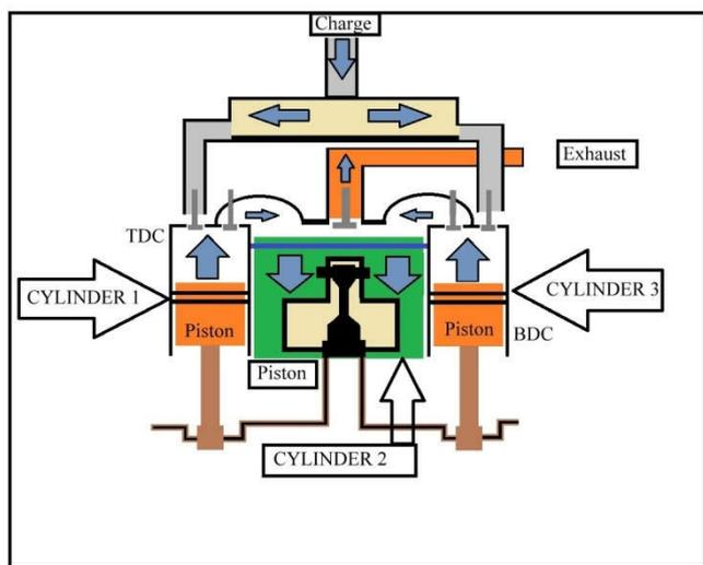
**Figure 1. Five stroke engine with three cylinders**
