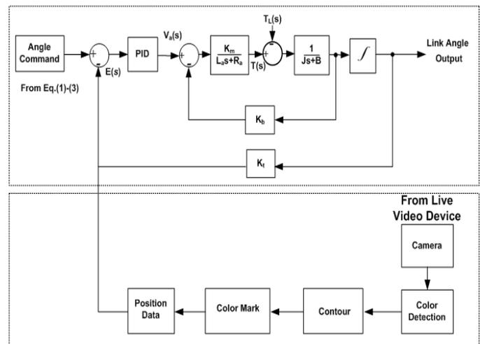
Fig. 3. The position tracking control system using the open CV
