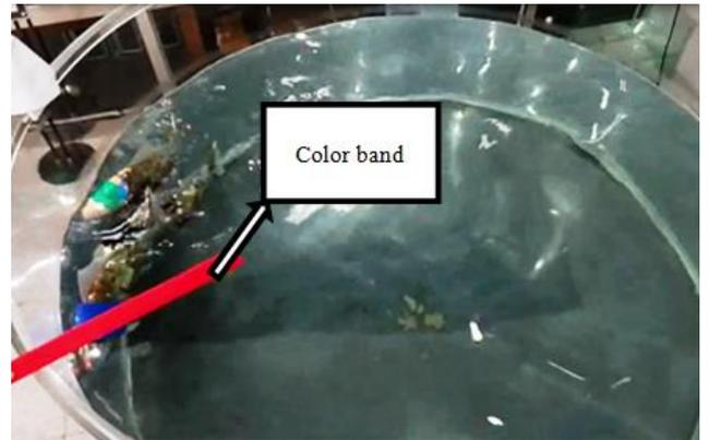
Fig. 10. The color mark tracking control of robot fish
