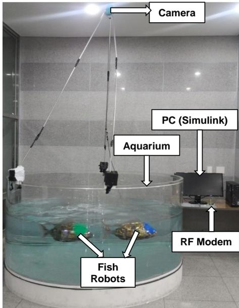
Fig. 7. The realization of robot fish using Open CV
