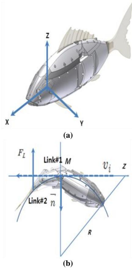
Fig2.(a) The axes of the robot fish, (b) The link angle rotation in the aquarium
