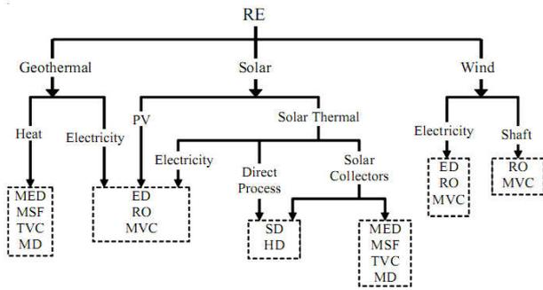
**Fig1. Technological Combinations of Conjunction of Renewable Energy with Water Purification Technologies**
