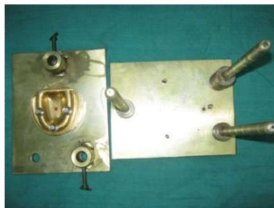
Fig. 2. Master model with impression zig apparatus
