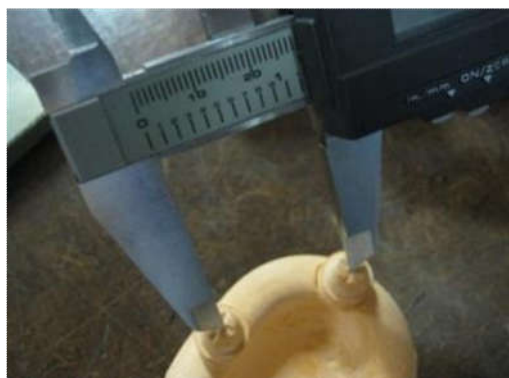
Fig. 7. Dimensions measured with vernier caliper
