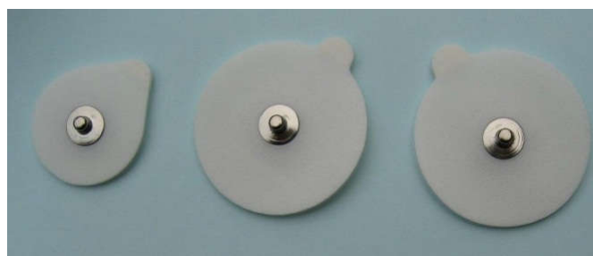
Fig.2. Electrodes used for ECG signal measurement
