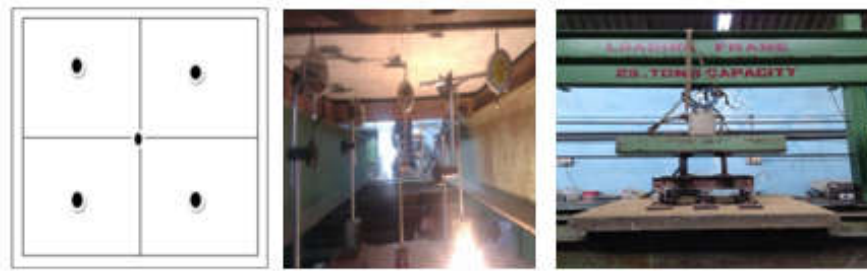
Fig.6. Layout and positioning of dial gauges, Test setup
