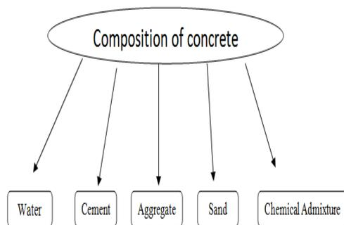
Fig 1. Composition of concrete
