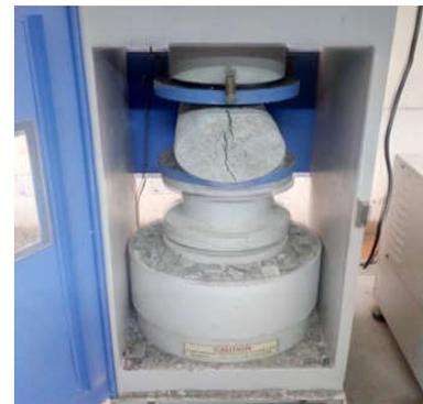
Fig.9. Concrete cylinder with crack
