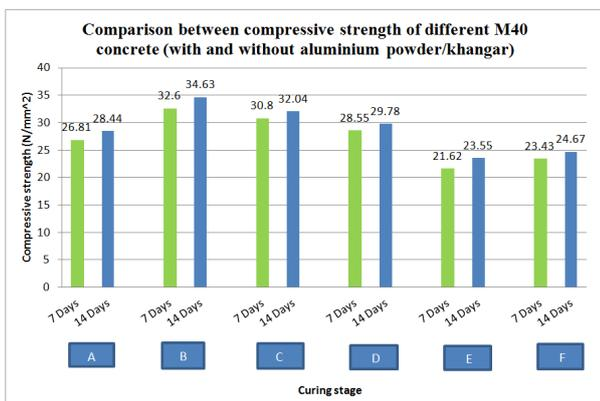
Fig. 12. Graph for comparison between compressive strength of different M40 concrete (with and without aluminium powder/khangar)
