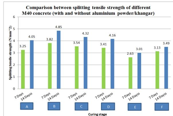
Fig.13. Graph for comparison between splitting tensile strength of different M40 concrete (with and without aluminium powder/khangar)
