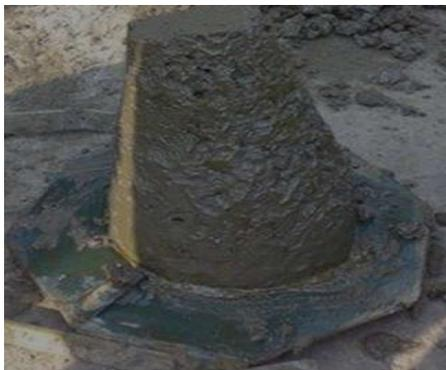
Fig. 5. Slump cone of concrete
