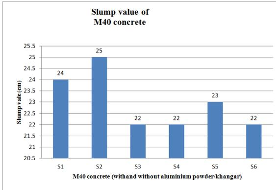
Fig. 11. Graph for slump values of M40 concrete
