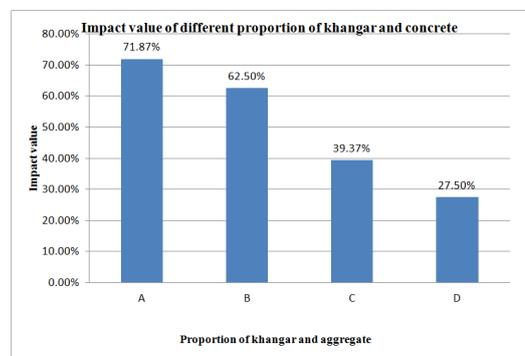
Fig 10 : Graph for impact value of different proportion of khangar and concrete
