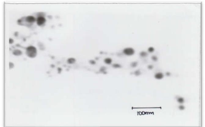
Fig. 5b. Shows mostly spherical particles of SNPsCMcFE, size 100 nM, (TEM, 19300X, 19 bar)
