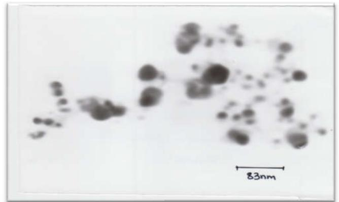
Fig. 5a. Shows Spherical SNPs of size 100 nM, (TEM at magnification 19300X, 19bar)
