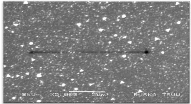
**Fig. 6a.** Shows different shape of SNPs mostly the spherical and triangular, hexahedral, cuboidal, size scale 5 µm (SEM, 5,000X, 8KV, scale)
