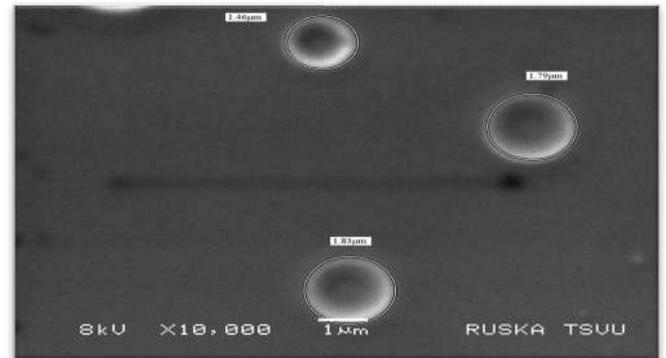
**Fig. 6b.** Shows spherical particles of SNPs coated with McFE, average size 1.93 µm, SEM, 5000 X, 8KV)
