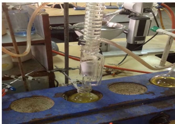
Fig. 2. A setup of Soxhlet apparatus
