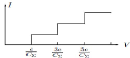
Figure 27(b). V-I Characteristics of the asymmetric junction SET
