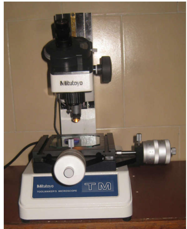
Figure 5. Travelling microscope (Mitutoyo, Japan)
