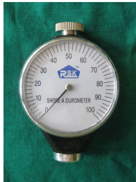
Figure 6. Shore - A Durometer (RSK Co., Taiwan)
