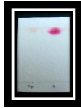
Fig. 9. TLC of standard and crude IAA S- stands for Standard IAA, Tip- stands for Crude sample
