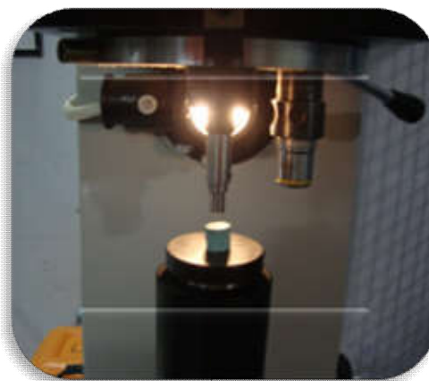
Fig.5. Making indentation with Vickers machine hardness measuring machine
