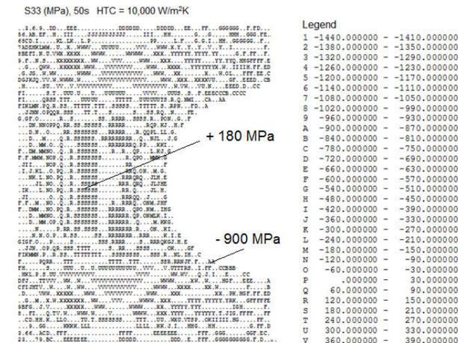
Fig. 10. Hoop stresses distribution in MPa in the roller (see Fig. 2) at the moment 50 sec when direct convection quenching with heat transfer coefficient equal 10,000 W/m<sup>2</sup>K
