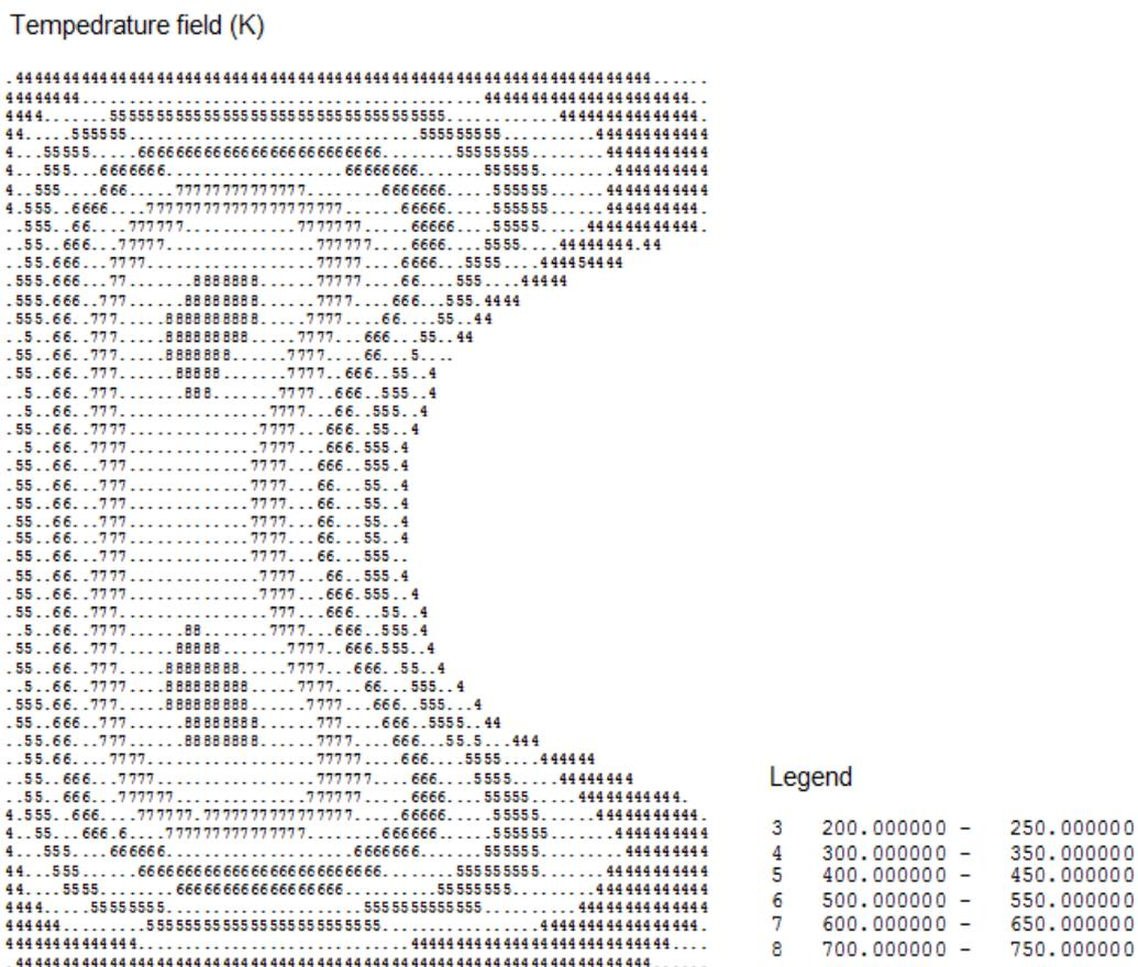
**Fig. 4. Temperature field in °K in the roller (see Fig. 2) at the moment 50 sec when direct convection quenching with heat transfer coefficient equal  $10,000 W/m^2K$**
