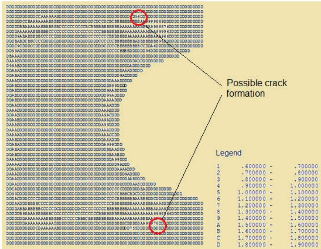
Fig. 6. Area in the roller where micro- cracks can appear at the moment 50 sec when direct convection quenching with a heat transfer coefficient equal to 10,000 W/m<sup>2</sup>K
