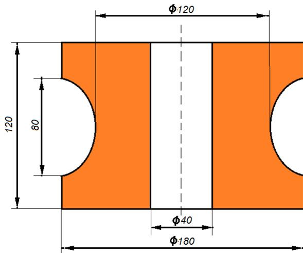
Fig. 2. Drawing of a roller used for FEM calculations
