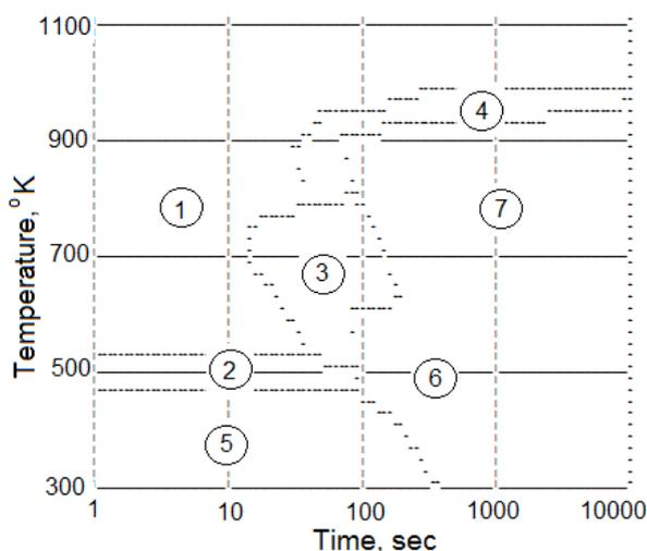
Fig. 3. CCT diagram used for FEM calculations: 1 is austenite; 2 is martensite; 3 is bainite; 4 is pearlite; 5 is martensite after full transformation; 6 is bainite after full process transformation; 7 is pearlite after full process transformation
