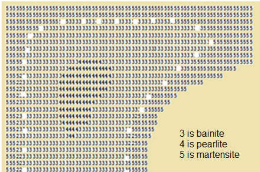
Fig. 5 Micro- structure distribution in the section of the roller at the moment 50 sec when direct convection quenching with a heat transfer coefficient equal to 10,000 W/m<sup>2</sup>K: 3 is bainite; 4 is pearlite; 5 is martensite
