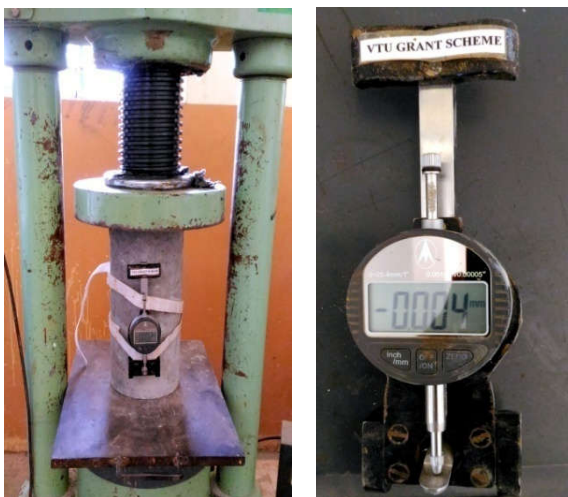
Fig.1. Measuring Strain in CTM Using Extensometer
