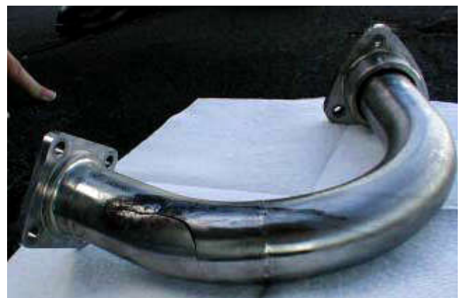
Photo 2. Air Transat 236, fuel pipe crack (AAPID, 2004, p. 17)
