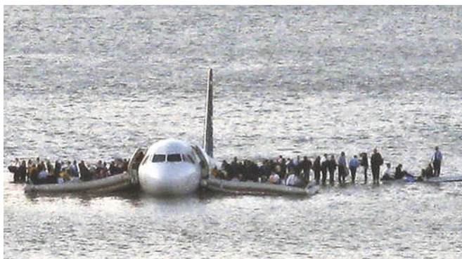
Photo 3. US Airways Flight 1549, aircraft on Hudson River, with occupants on the wings and slide/rafts after the evacuation (NTSB, 2010, p. 5)
