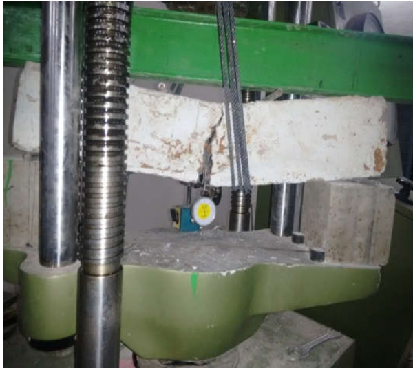
Fig 2(b). Tested beam in flexure
