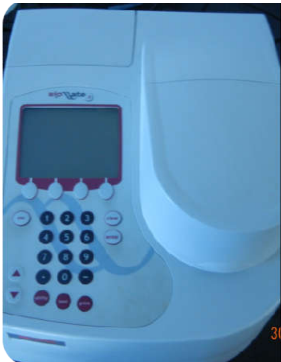
Figure 2. Spectrophotometer method for charecterization of nanoparticles
