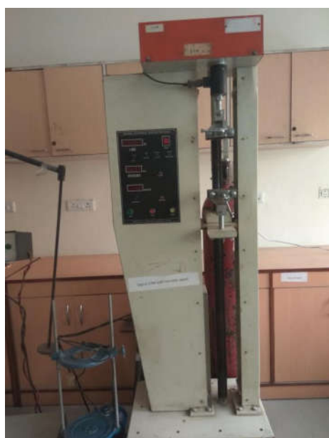
Fig. 4. Universal testing machine used for measuring fracture resistance
