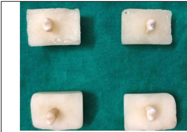
Fig.4. Restored samples mounted on acrylic blocks
