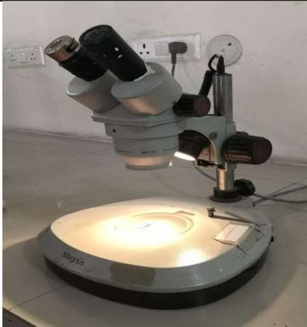
Fig. 6. Stereomicroscope
