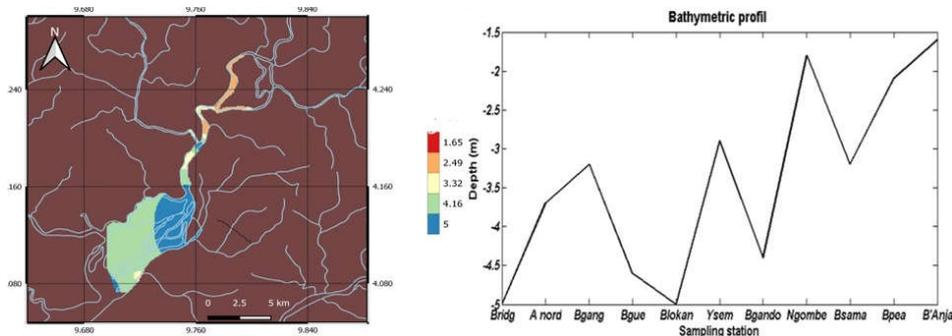
Figure 3: Evolution of depth in the upper section of the Cameroon estuary
