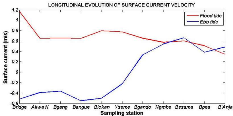
Figure 4: Surface current evolution along the Wouri-Nkam section of the Cameroon estuary
