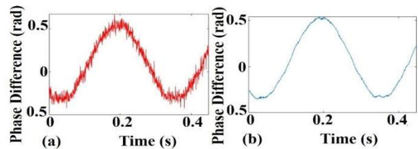
Figure 5. Original and denoised time domain signals
