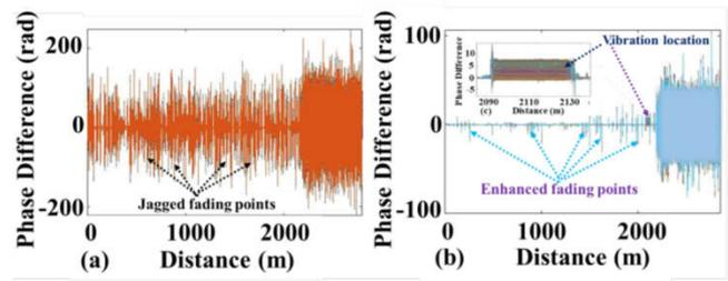
Figure 4. Original and denoised phase trace
