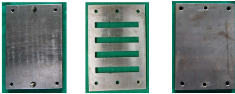
Fig.1. Custom made stainless Steel mold (lower, middle and upper member), V shaped notch
