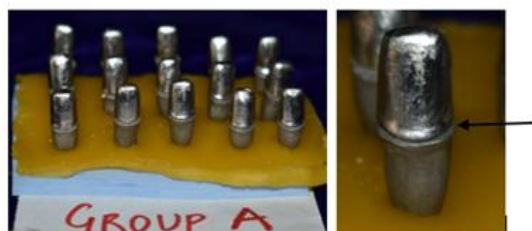
Figure 7 :Group A : 15DMLS copings extending up to gingivo-axial line angle offinish line.
