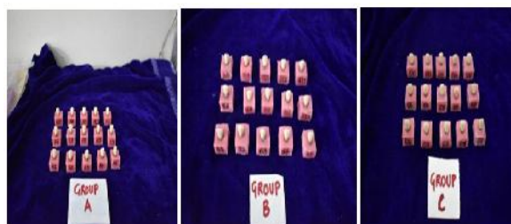
Figure 11. The 45 specimens were embedded in acrylic resin blocks followed by cementation of the ceramo-metal crowns to respective dies using resin modified glass ionomer agent. 15 specimens each for groups A,B,C
