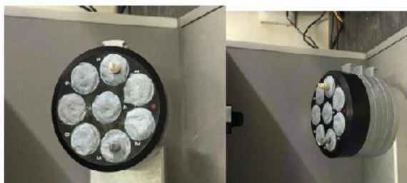
Figure 6 Scanning of metal dies for DMLS coping
