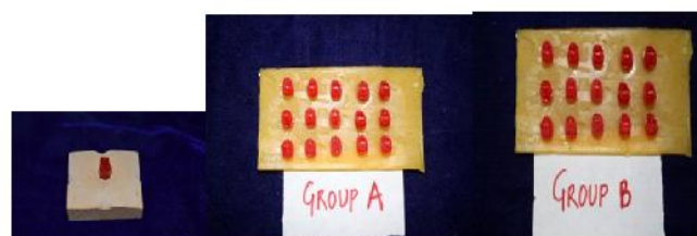
Figure 4 : A resin die (poly methyl methacrylate) of the prepared ivory tooth was fabricated, group A and B – 15 specimens each
