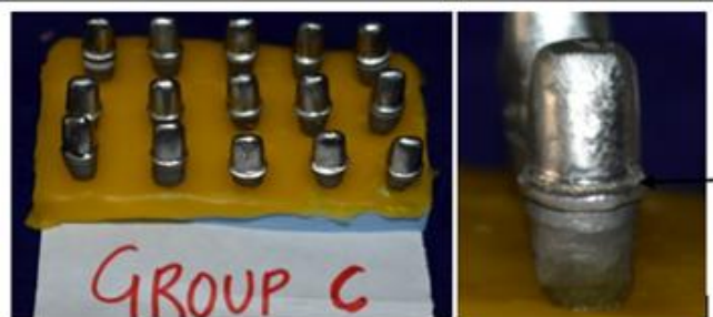
Figure 10. Group C : 15 DMLS copings having 0.4mm wide labial metal collar. Step 5- Modification of the prepared ivorine tooth for fabrication of dies and copings for Group C:
