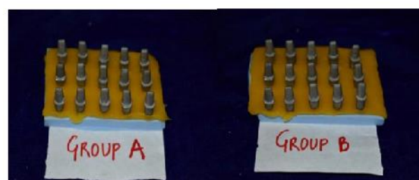
Figure 5 : The 30 metal dies (group A and B) were casted in Ni-Cr alloy according to the standard casting protocol in conventional method
