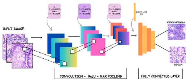
Figure 4. Proposed dcnn model's architecture
